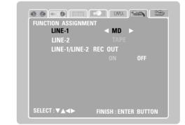
Use the  $\blacktriangle$  and  $\triangledown$  cursor buttons to select the item to be set, then use the  $\blacktriangleleft$  and  $\blacktriangleright$  cursor buttons to make the settings.
